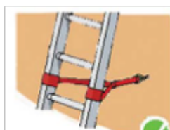
Figure 7 - Tying near the base of the ladder
