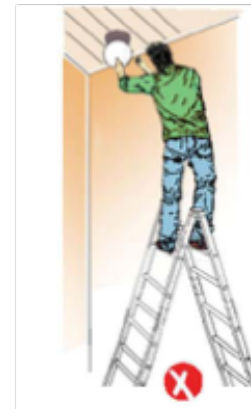
Figure 3 - never straddle a stepladder
